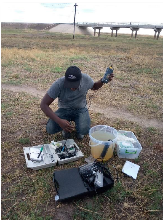
Figure 1: Mulema taking onsite measurement of physiochemical parameters from a perennial surface water body in the dry season
