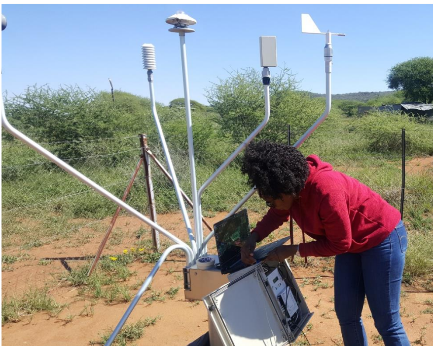
Figure 1: Meteorological data download at the Ranaka automated Weather Station
